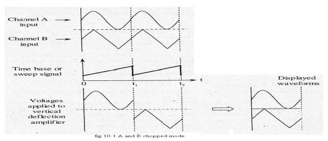
segments are so small that the trace of low frequency signal appears to be a continuous waveform. Hence, chop mode display is usually preferred for low frequency signals.
