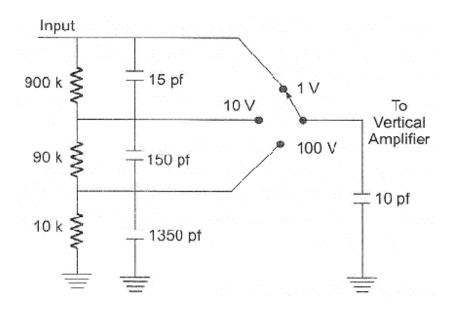
fig 8.2 Simple Compensated Attenuator
