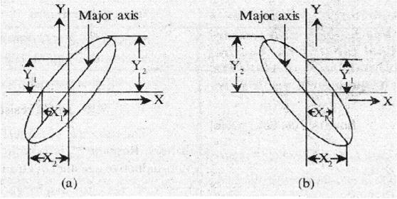
fig 6.1 Determinig Angle of phase shift
