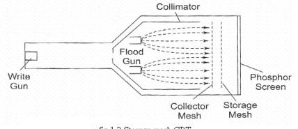
Since the storage mesh makes use of secondary emission, between the first and second crossover more electrons are emitted than are absorbed by the material, and hence a net positive charge results.
