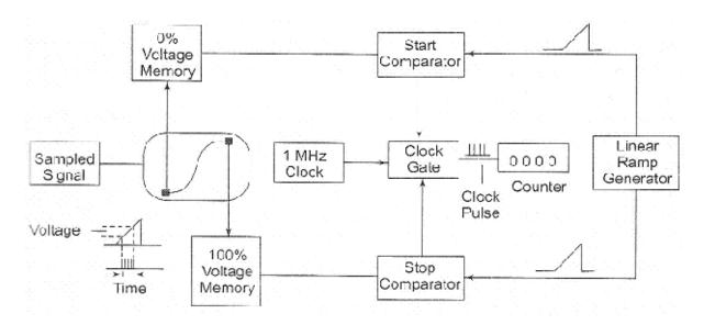
fig 9.2 Voltage to time conversion
