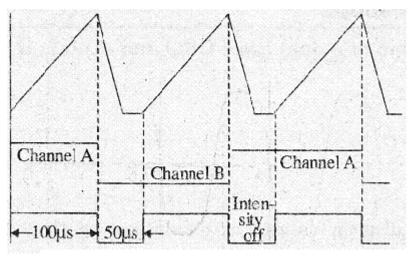
fig 2.2 Wae form of Dual trace oscilloscope in Alternate mode
