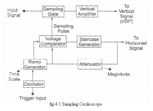
Fig 4.1 shows a block diagram of a sampling oscilloscope. The input is applied to the sampling gate. The input waveform is sampled whenever a sampling pulse opens the sampling gate. The sampling must be synchronized with the input signal frequency. The signal is delayed in the vertical amplifier, allowing the horizontal sweep to be initiated by the input signal. The waveforms are shown in fig 4.2
