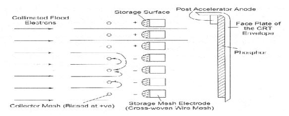
fig 1.3 Display of stroed charge pattern on a mesh
